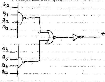
nand4:  $t_{df} = R_n C_g \cdot 4(4+2) = 24R_n C_g$  ;  $t_{dr} = R_p C_g (4+2) = 6R_p C_g$
