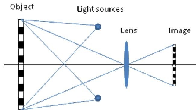
Figure 6. Experimental setup for front-light illumination.
