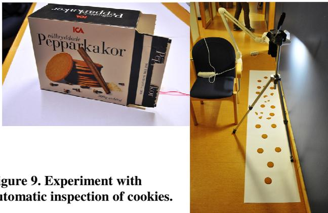
Figure 9. Experiment with automatic inspection of cookies.
