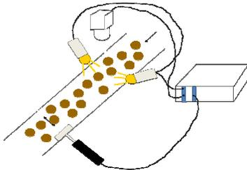
Figure 8. Machine vision system for inspection of cookies.
