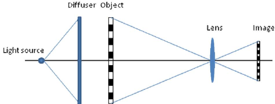
Figure 5. Experimental setup for back-light illumination using a diffuser.
