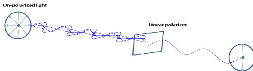
Figure 3. Linear polarization of light using polarization filter
