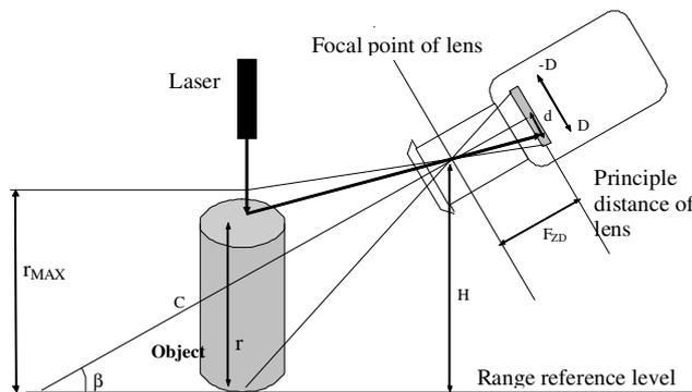
Figure 12. Principle sketch for laser triangulation.
