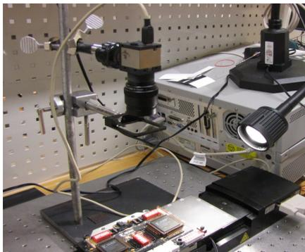
Figure 4. Setup for imaging of circuit board.
