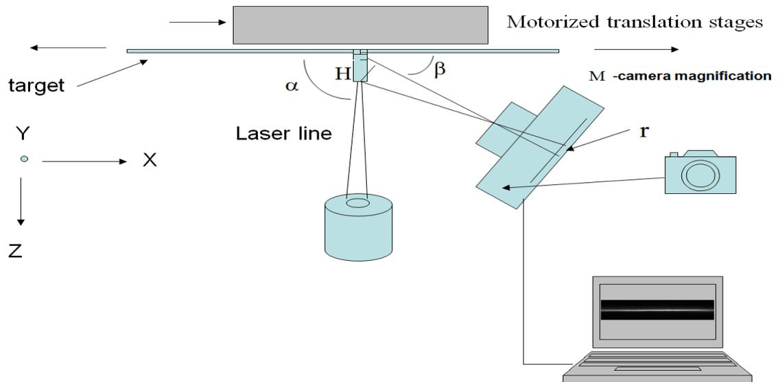
Figure 14. Schematic picture of motorized laser scanner.
