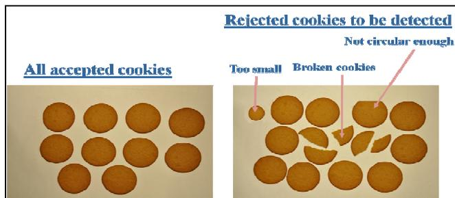
Figure 10. Example of accepted and rejected cookies.
