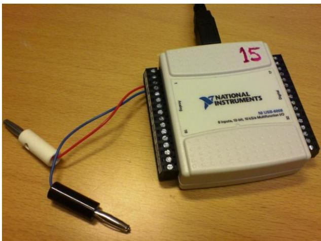
Figure 3.2. DAC-ADC unit to be used with LabVIEW.
