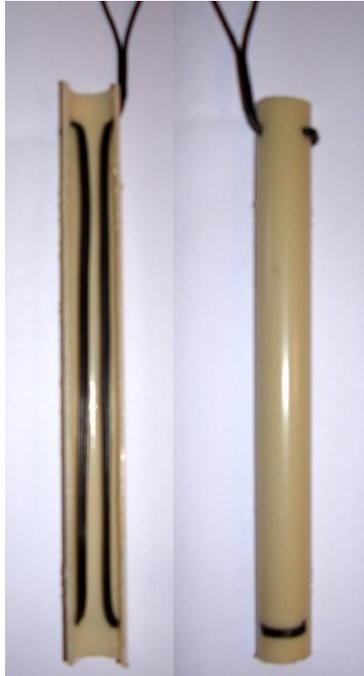
Figure 1.3 – Cross-section of the sensor seen from the inside and the outside
