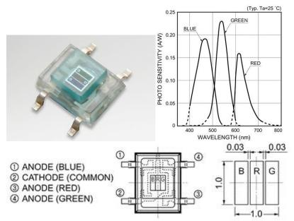
Use the available setup where a RGB sensor is connected to a DAQ Unit (NI USB-6009) via a preamplifier. Only the "R" and the "B" signal are connected. Use LabView to make software for temperature measurements.
