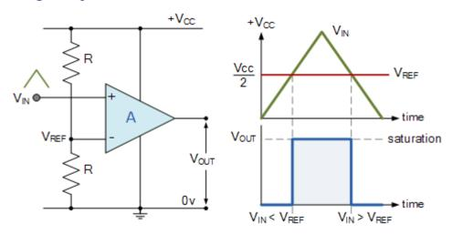
In this non-inverting configuration, the reference voltage is connected to the inverting input of the operational amplifier with the input signal connected to the non-inverting input. To keep things simple, we have assumed that the two resistors forming the potential divider network are equal and: R1 = R2 = R. This will produce a fixed reference voltage which is one half that of the supply voltage, that is Vcc/2, while the input voltage is variable from zero to the supply voltage.
