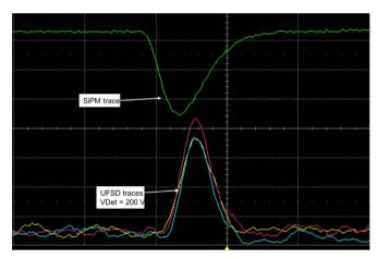
**Fig. 5.** Screenshot of one event, showing the signals of 3 UFSD biased at 200 V and the SiPM at 28 V. Each horizontal division corresponds to 2 ns, while each vertical division is 100 mV.
