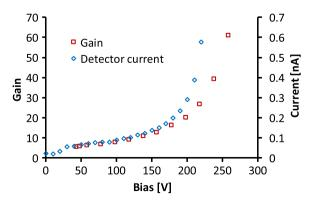
Fig. 1. Bias dependence of the leakage current and the signal gain for a 45  $\mu m$ -thick UFSD sensor with an area of 1.7 mm². The gain determination is subject to an overall scale uncertainty of 20%. The similar exponential behaviour of gain and sensor current below 200 V bias is due to the common charge multiplication mechanism.
