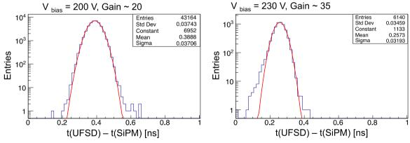
Fig. 7. Time difference UFSD-SiPM at 2 different UFSD bias voltages: 200 V with sigma=37 ps, and 230 V with sigma=32 ps.
