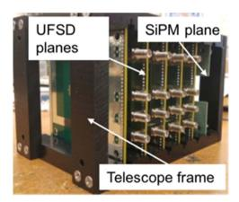
**Fig. 4.** Beam test frame showing four UFSD boards and the trigger counter. Alignment was assured with four rods (not shown) going through aligning holes in the four corners of the boards and the frame.
