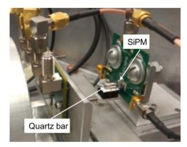
Fig. 3. Trigger counter configuration shown in the  $\beta$ -source: the 10 mm long quartz bar mounted on the SensI. SiPM evaluation.
