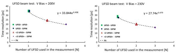
Fig. 8. Timing resolution for: single UFSD (N=1) obtained from the UFSD-SiPM and UFSD-UFSD time differences; averaged pairs of UFSD (N=2) and average of 3 UFSD (N=3) for bias voltages of (left) 200 V and (right) 230 V.
