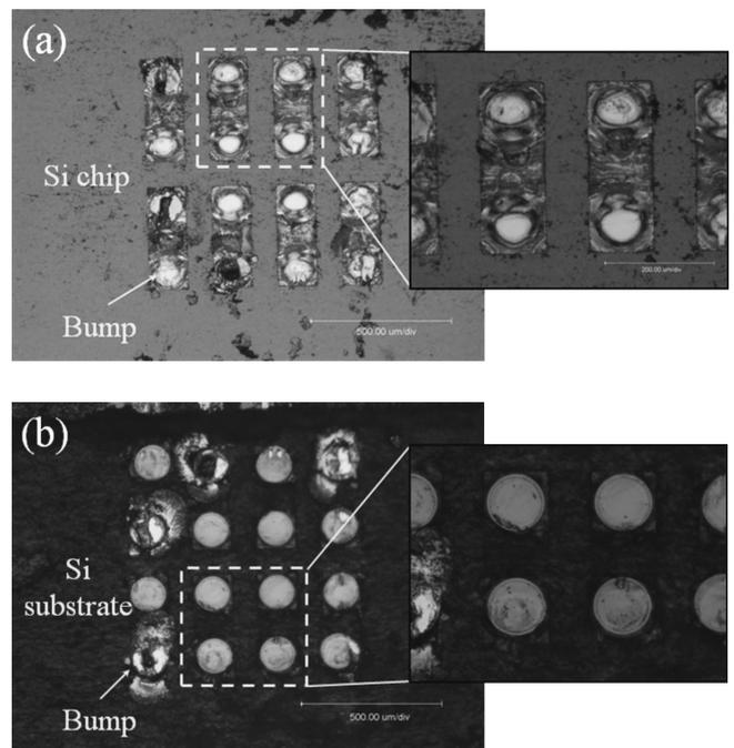
Fig. 10 Fracture surfaces of (a) a chip and (b) substrate after TS ACF flip-chip bonding with a 433 K bonding temperature and a 0.5 s bonding time (TSB-4).
