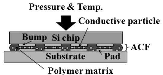
Fig. 1 Schematic diagram of typical thermo-compression (TC) ACF flip-chip bonding.
