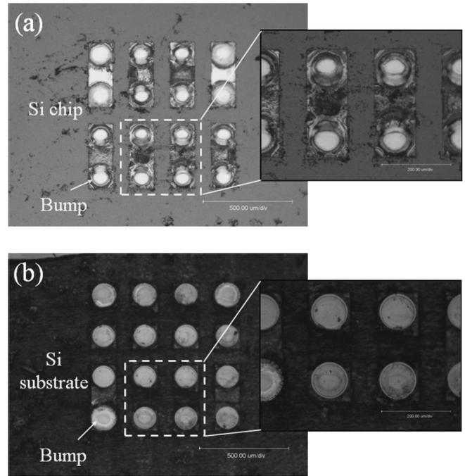
Fig. 9 Fracture surfaces of (a) a chip and (b) substrate after TC ACF flip-chip bonding (TCB).
