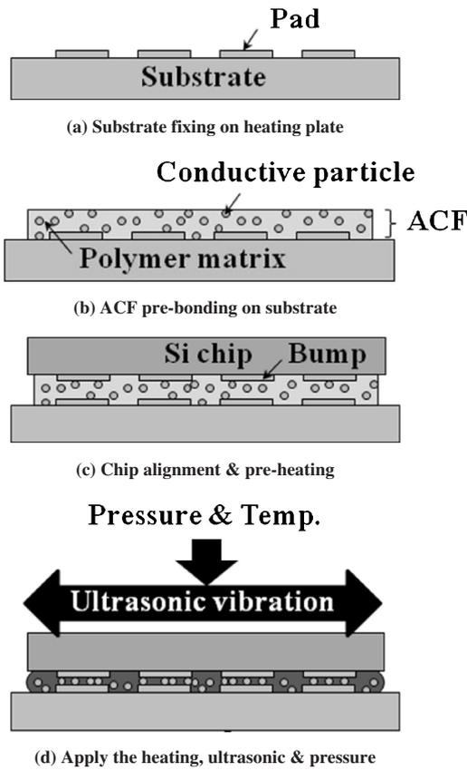
Fig. 4 TS ACF flip-chip bonding process.
