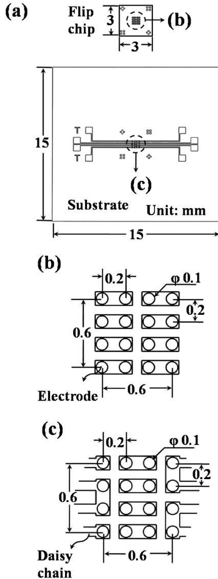
Fig. 2 Configuration of (a) the flip-chip and substrate and the electrode pattern of (b) the flip-chip and (c) substrate.
