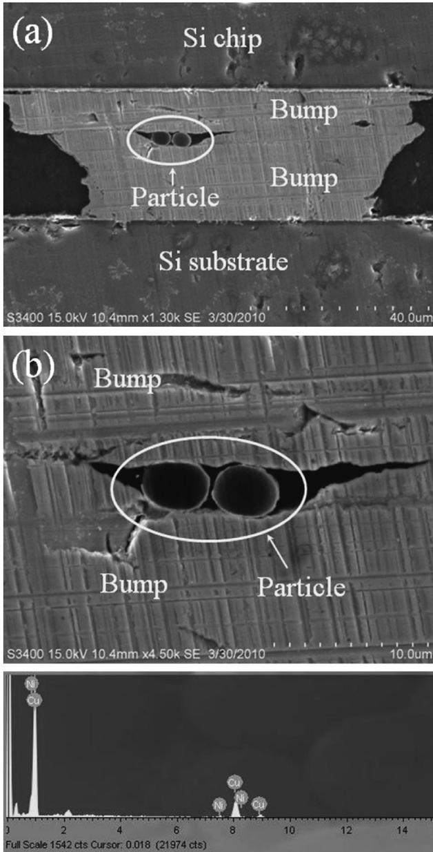
Fig. 6 SEM-EDS analysis of the flip-chip assembly bonded by the conventional TC ACF bonding process (TCB). (a) SEM micrograph and (b) EDS analysis.
