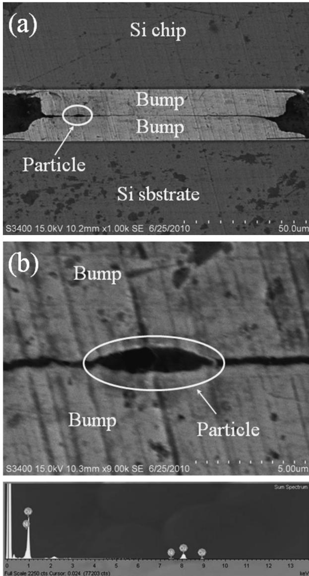
Fig. 8 SEM-EDS analysis of the TS flip-chip assembly with 0.5 s (TSB-4) for bonding time at 433 K for bonding temperature. (a) SEM micrograph and (b) EDS analysis.
