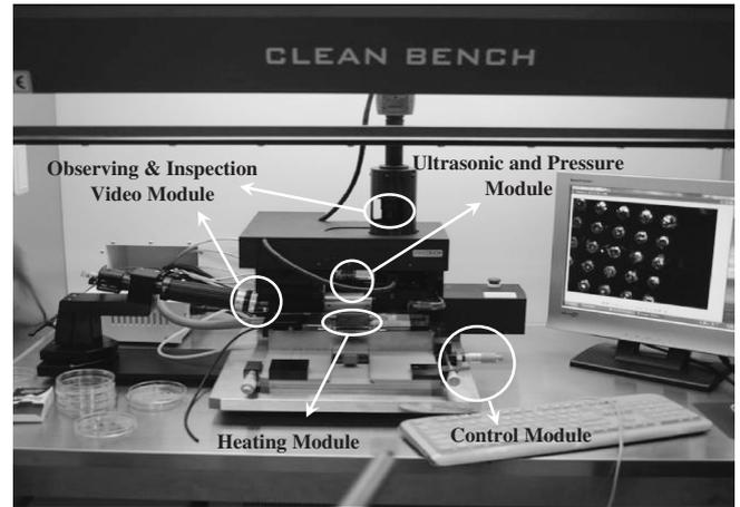
Fig. 3 Experimental setup for the TS ACF flip-chip bonding test.
