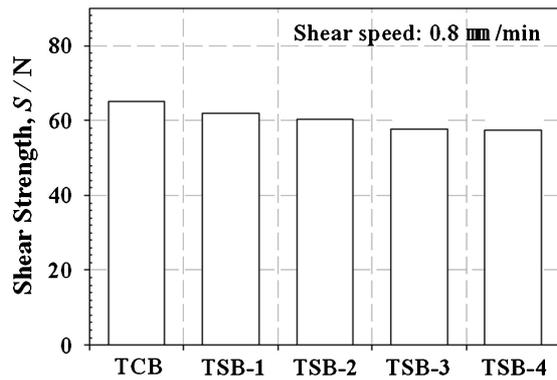
Fig. 11 Shear strengths of TC and TS ACF flip-chip assemblies.
