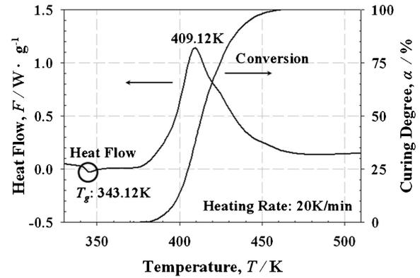
Fig. 5 DSC results at a heating rate of 20 K/min.
