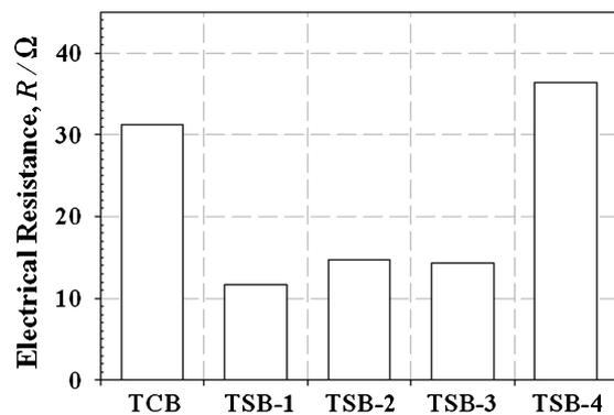
Fig. 12 Total daisy-chain electrical resistances of TC and TS ACF flip-chip assemblies.
