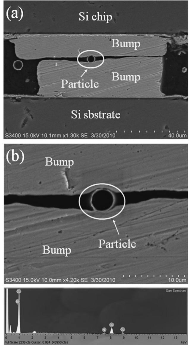
Fig. 7 SEM-EDS analysis of the TS flip-chip assembly with 0.5 s (TSB-2) for bonding time at 453 K for bonding temperature. (a) SEM micrograph and (b) EDS analysis.
