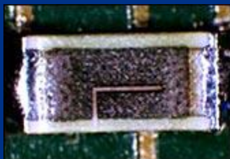
'L' cut into a thick film resistor
