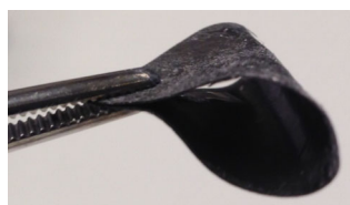
Figure 4 Bent nanographite–NFC film after operation in a SC.
