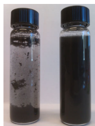
Figure 5 Stability of nanographite dispersions without NFC (left vial) and with 10% NFC (right vial).
