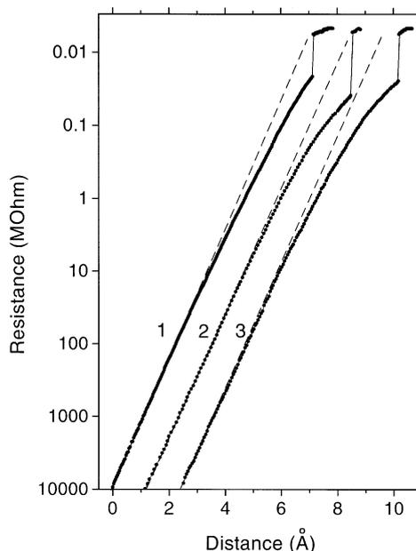
Fig. 3. Deviation of  $R(z)$  curves from exponential behavior for MCBJ containing magnetic particles: 1.—Ni; 2.—Fe; 3.—Co.
