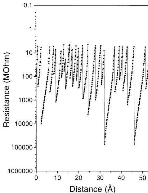
Fig. 5.  $R(z)$  dependence for Fe MCBJ containing small magnetic particle at elevated bias voltage  $V_b = 1100$  mV.
