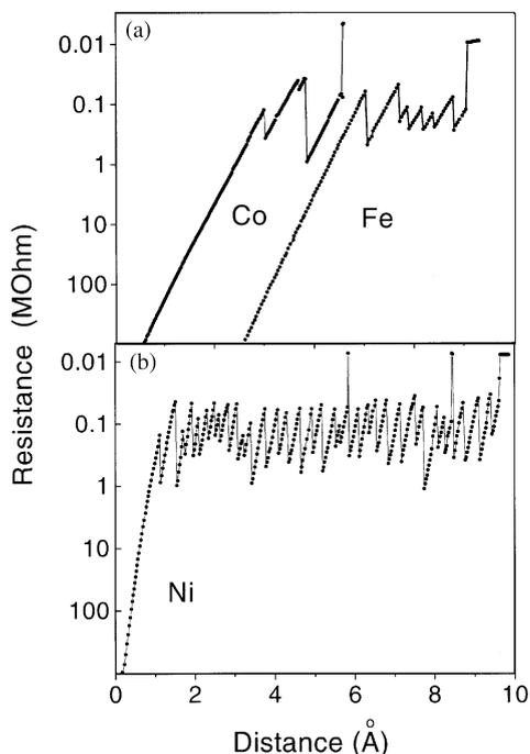
Fig. 4. Jump-like behavior of  $R(z)$  at close electrode separation for MCBJ involving nanoparticle: (a)—Fe and Co tunnel junction; (b)—Ni MCBJ. All curves were recorded at bias voltage of 10 mV.
