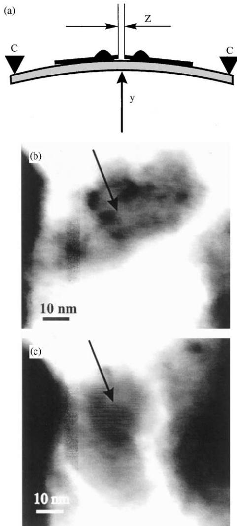
Fig. 1. (a) Design and principle of a mechanically controllable break junction. A bending force causes a vertical displacement  $y$ , which leads to a distance  $z$  between the electrodes. For clarity, all distances have been exaggerated. (b), (c) TEM image of Ni nanoparticle (indicated by an arrow) confined between electrodes of MCBJ.
