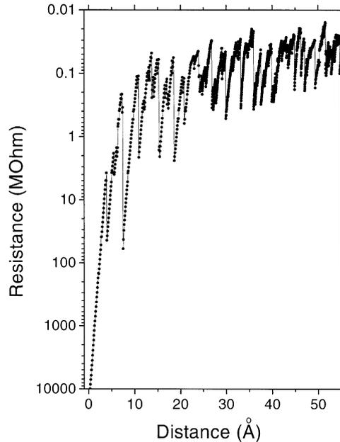
Fig. 6.  $R(z)$  dependence for usual Co MCBJ (without magnetic particles between electrodes). The abrupt jumps of decreasing amplitude in junction resistance related at initial step to the field desorption of weakly bound adatom and then to the field induced diffusion of the surface atoms [24].
