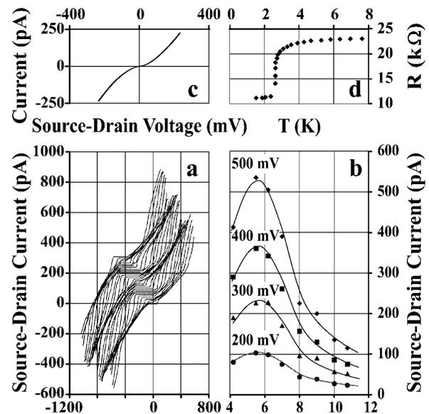
FIG. 3. (a) A set of  $I(V)$  curves taken at different gate voltages equally spaced in the region  $\pm 1100$  mV at 4.2 K. (b) Temperature dependence of the tunneling current at different biases for the open state of the transistor; (c) an  $I(V)$  curve of a single tunneling gap. (d) Superconducting transition in the leads.
