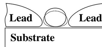
FIG. 4. The cluster tends to restore spherical symmetry at high temperature as a result of a phase transition. This leads to wider tunneling gaps above the transition temperature.
