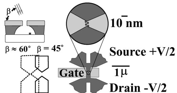
FIG. 1. Left—tuning the constriction width: starting from  $\beta = 45^\circ$  the tilt was incremented stepwise narrowing the gap between the leads by 10 nm at each step. After each step 2 nm of material was deposited and the sample conductivity was measured to check if a connection had been made. Right—resulting sample geometry. Substrate—oxidized silicon; gate—oxidized aluminum.
