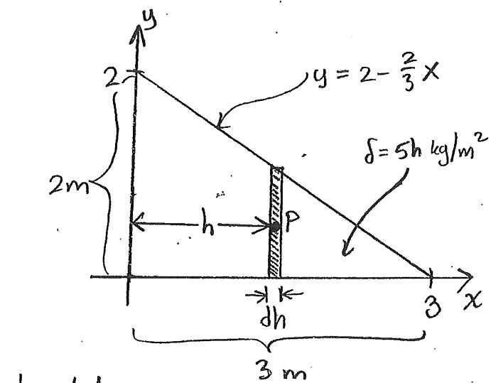
$$dA = \underbrace{\left(2 - \frac{2}{3}h\right)}_{\text{höjd}} \underbrace{dh}_{\text{bredd}}$$
