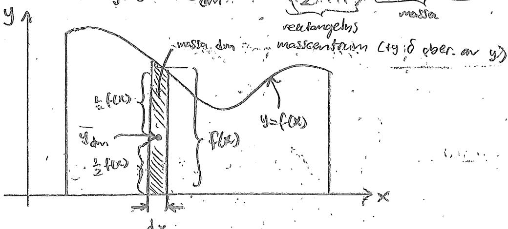
$$\bar{x} = \frac{M_{x=0}}{m} \quad \text{och} \quad \bar{y} = \frac{M_{y=0}}{m} \quad \text{gaf masscentrum } (\bar{x}, \bar{y})$$
