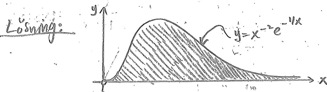
$$\text{Arealen: } A = \int_0^{\infty} x^{-2} e^{-1/x} dx = \underbrace{\int_0^1 x^{-2} e^{-1/x} dx}_{= I_1} + \underbrace{\int_1^{\infty} x^{-2} e^{-1/x} dx}_{= I_2}$$
