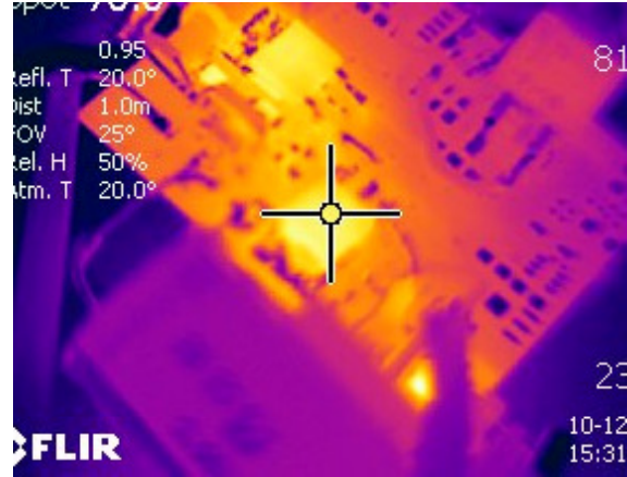
Figure 10. Temperature profile of MOSFET
