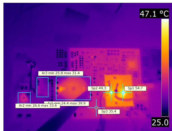
Fig.10. Thermal profile of LLC DC-DC converter at f_{sw} of 3.3MHz and P_{load} of 45W at V_{in}^{min} of 127V_{DC} at an ambient of 25^{\circ}C
