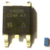
Fig.1 Size comparison of 200V Si (DPAK) –left and GaN (LGA) - right enhancement mode MOSFET
